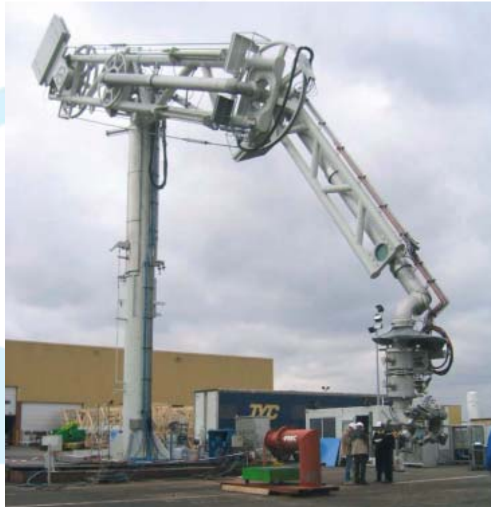
Loading arm liquefied natural gas
